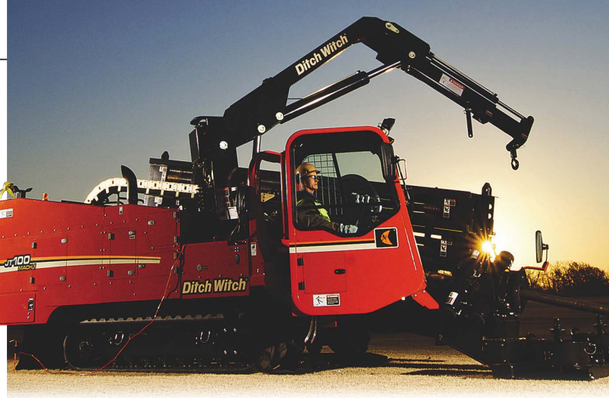
With 100,000 pounds of pullback and 12,000 pounds-per-foot of torque, the 268-horsepower JT100 is the largest Ditch Witch horizontal directional drill, built for both long-range bores and large-diameter pipe installations. There's plenty of power, says Ditch Witch, for an optional onboard crane and anchor system.
