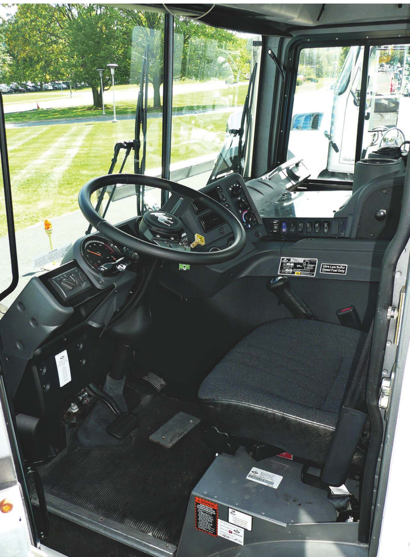
Lower engine cover makes the interior seem more spacious, and there's now sufficient leg and belly room for the driver.
